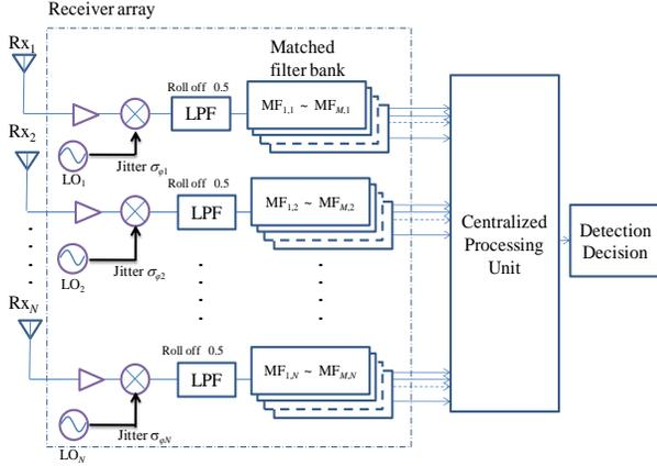
Fig. 7. Phase jitter in the MIMO radar receiver array.
