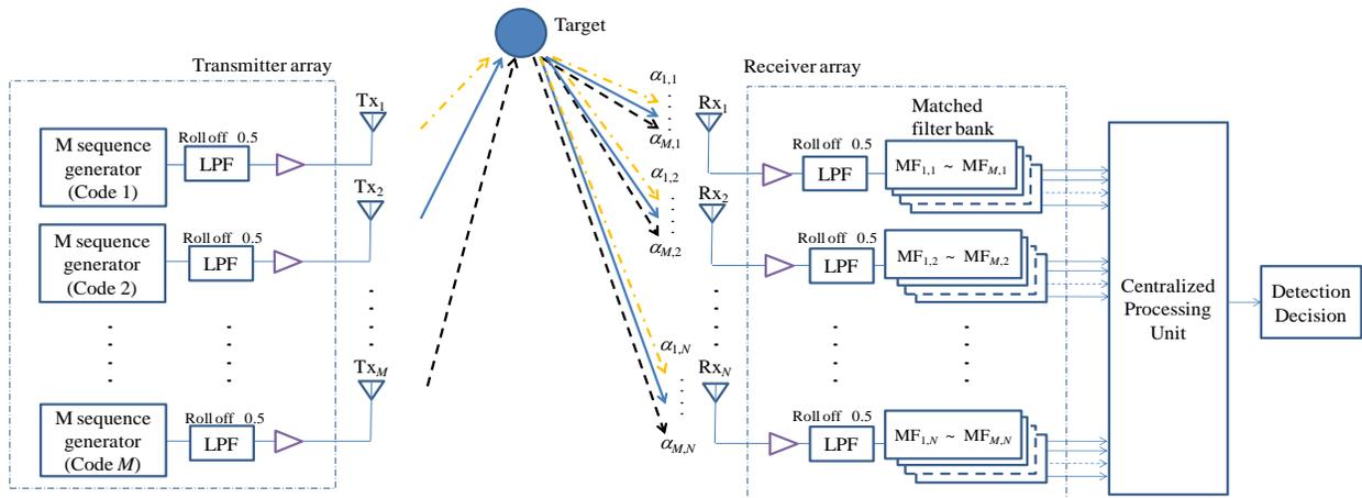
Fig. 1. MIMO radar system diagram.
