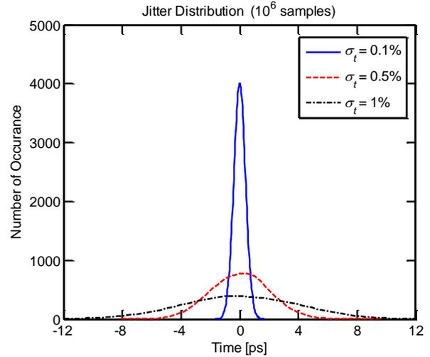
Fig. 3. Modeled jitter distribution with different values of  $\sigma_t$ .
