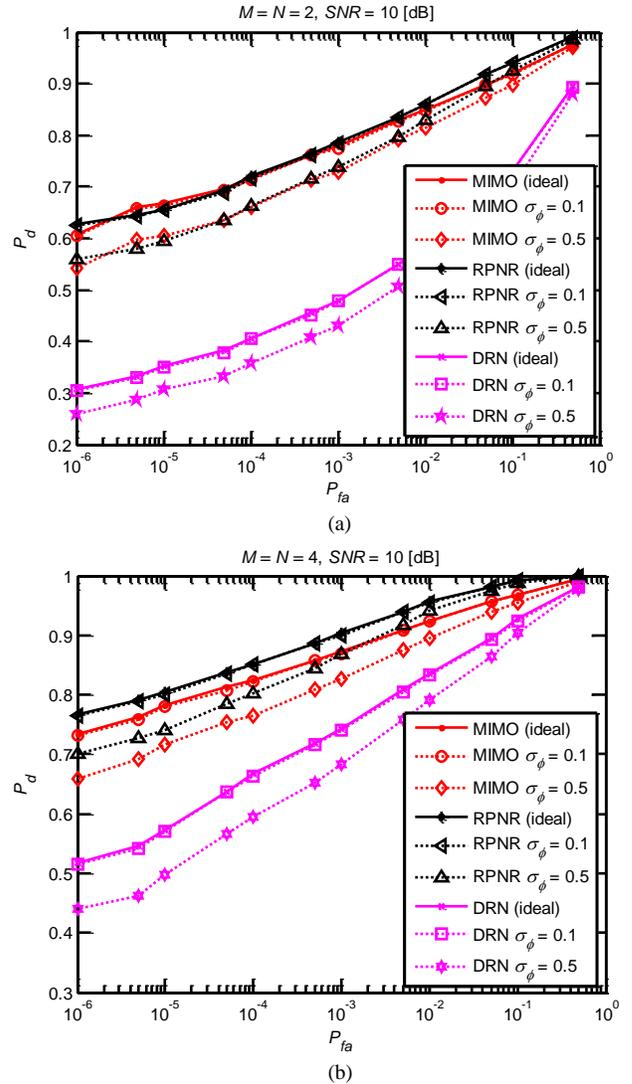
Fig. 9. Receiver operating curves of the simulated MIMO radar systems with presence of severe phase jitter: (a)  $2 \times 2$  and (b)  $4 \times 4$  configurations.
