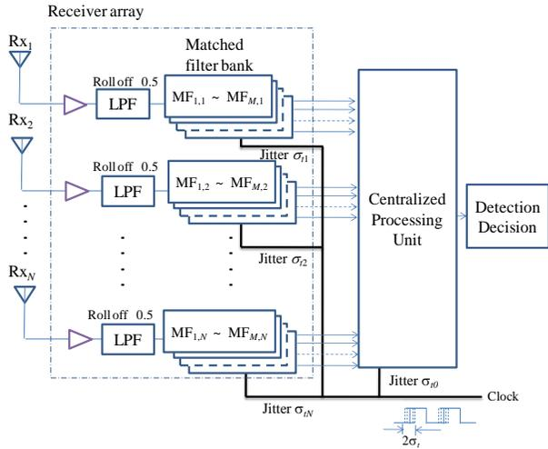
Fig. 2. Timing jitter in the MIMO radar receiver.
