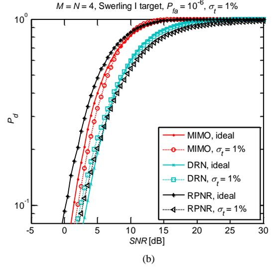
Fig. 6. Probability of detection under jitter influence in a 4x4 configuration: (a)  $\sigma_t = 0.1\%$  and (b)  $\sigma_t = 1\%$ .
