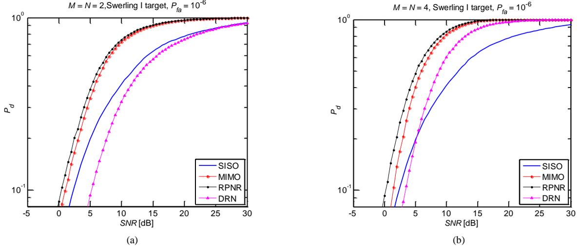
Fig. 4. Probability of detection of the simulated MIMO radar system in ideal cases: (a)  $2 \times 2$  and (b)  $4 \times 4$  configurations.
