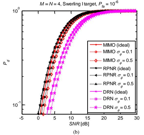
Fig. 8. Simulated probability of detection of MIMO radar system under phase jitter influence: (a) 2x2, and (c) 4x4 configurations.
