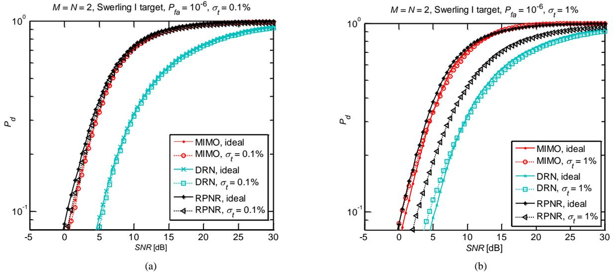
Fig. 5. Probability of detection under jitter influence in a  $2 \times 2$  configuration: (a)  $\sigma_t = 0.1\%$  and (b)  $\sigma_t = 1\%$ .
