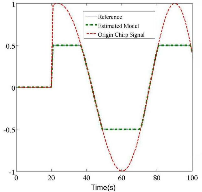
Fig. 6. Comparison of estimated model and reference model: saturation model
