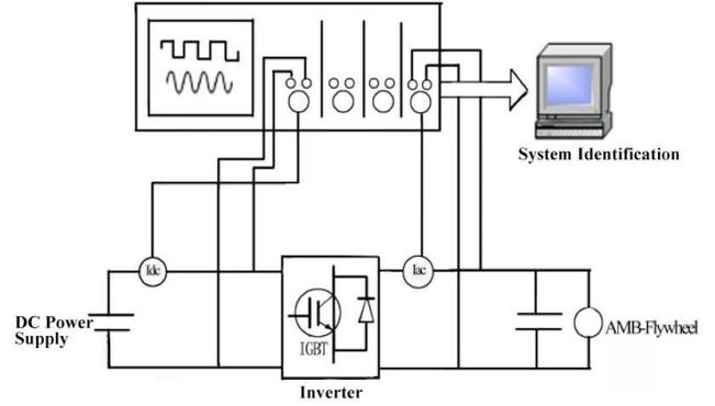
Fig. 8. Schematic of experimental setup for inverter modeling
