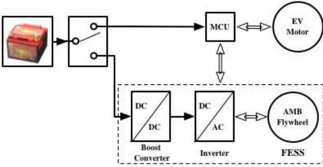
Fig. 1. AMB-FESS for EV Architecture
