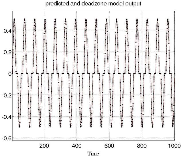
Fig.7. Outputs for predicted and selected deadzone models
