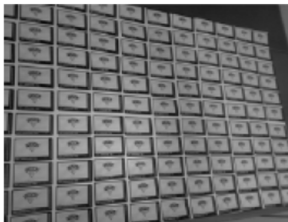
Fig. 3. Rear View of the Projecting Screen with NFC tags (Source [11])
