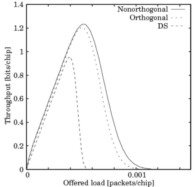
Fig. 6. Normalized throughput versus offered load ( $L_{p-info}=2520$ ,  $E_b/N_0=\infty$  [dB],  $K=200$ ,  $L_{signal}=128$ )
