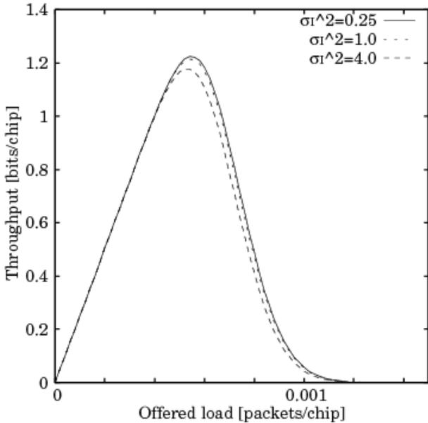
Fig. 8. Normalized throughput of our system versus offered load ( $L_{p-info}=2520$ ,  $M_{os}=32$ ,  $M_{con}=4$ ,  $E_b/N_0 = \infty$  [dB],  $K=200$ ,  $L_{signal}=128$ )
