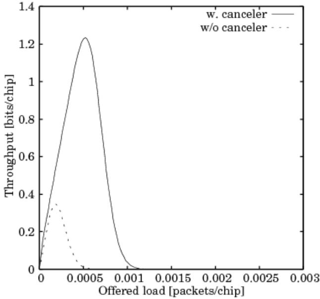
Fig. 4. Normalized throughput of our system versus offered load ( $L_{p-info}=2520$ ,  $M_{os}=32$ ,  $M_{con}=4$ ,  $E_b/N_0=\infty$  [dB],  $K=200$ ,  $L_{signal}=128$ )
