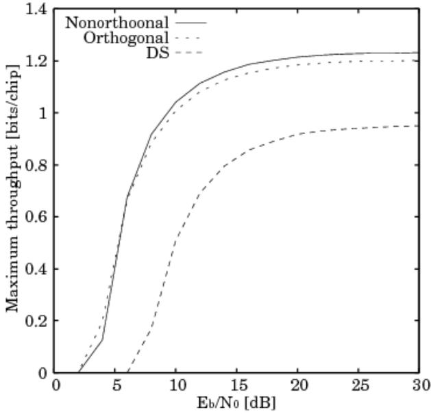
Fig. 7. Maximum throughput versus  $E_b/N_0$  ( $L_{p-info}=2520$ ,  $K=200$ ,  $L_{signal}=128$ )
