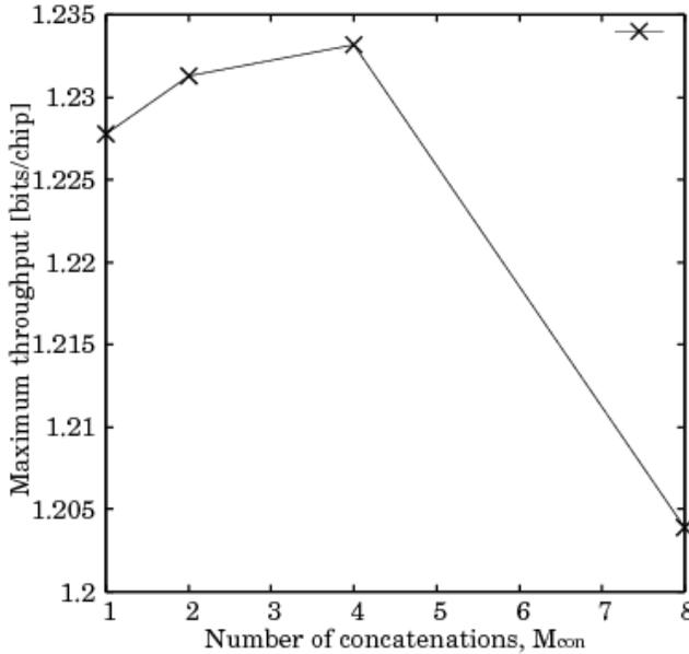
Fig. 5. Maximum throughput of our system versus number of concatenations ( $L_{p-info}=2520$ ,  $M_{os}=32$ ,  $E_b/N_0=\infty$  [dB],  $K=200$ )
