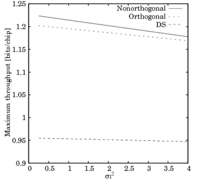
Fig. 9. Maximum throughput of our system versus  $\sigma_I^2$  ( $L_{p-info}=2520$ ,  $E_b/N_0 = \infty$  [dB],  $K=200$ ,  $L_{signal}=128$ )
