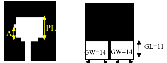
Figure 8: Structure of partial slotted ground antenna with addition of stair and stub.
