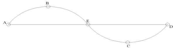
Consider the curved segment ABC in the above Fig. 3 we must have nodes at end point A, endpoint C and node at B. Also if ABCECD curved segment is considered in Fig.4, node should be present at A, B, C and D, where A and D are the end points and B and C are the points where a significant change in direction has occurred.
