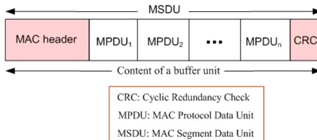
Figure 2. Frame structure of the BUMA protocol.
