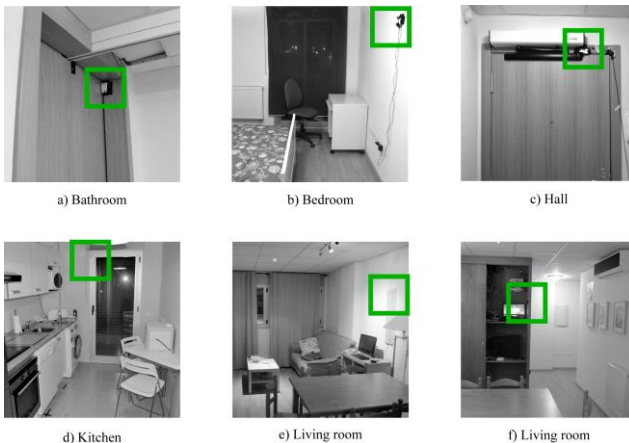
Fig. 8. Placement of presence sensors within a laboratory flat.
