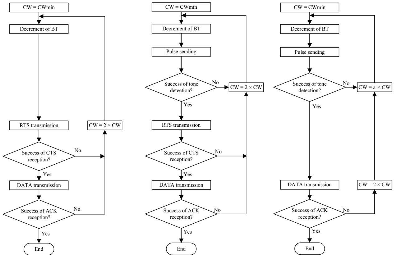
Fig. 3. Flowcharts of DMAC, RCA and the proposed protocols. (a) The DMAC protocol. (b) The RCA protocol. (c) The proposed protocol.
