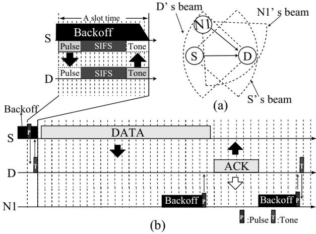
Fig. 5. An example of mitigating the directional hidden-node problem in the proposed protocol. (a) An scenario. (b) Time-domain expression.
