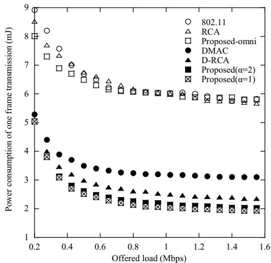
Fig. 10. Power consumption for one frame transmission as a function of the offered load at each node.
