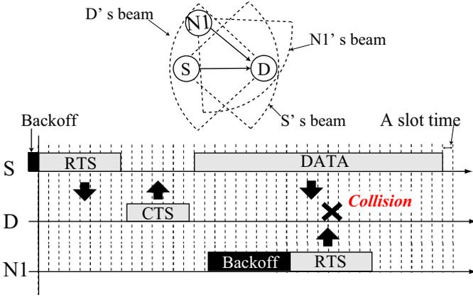
Fig. 1. An example scenario of the collision due to the directional hidden-node problem in the DMAC protocol.
