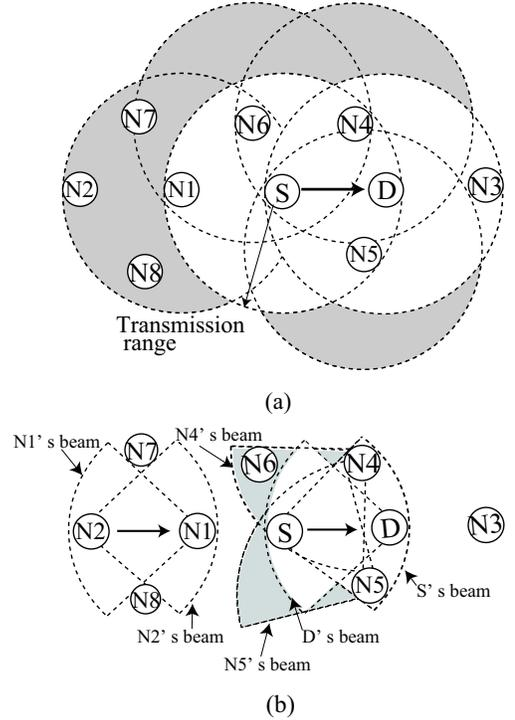
Fig. 2. Examples for exposed node increasing in the RCA and proposed protocols. (a) the RCA protocol (b) The proposed protocol.
