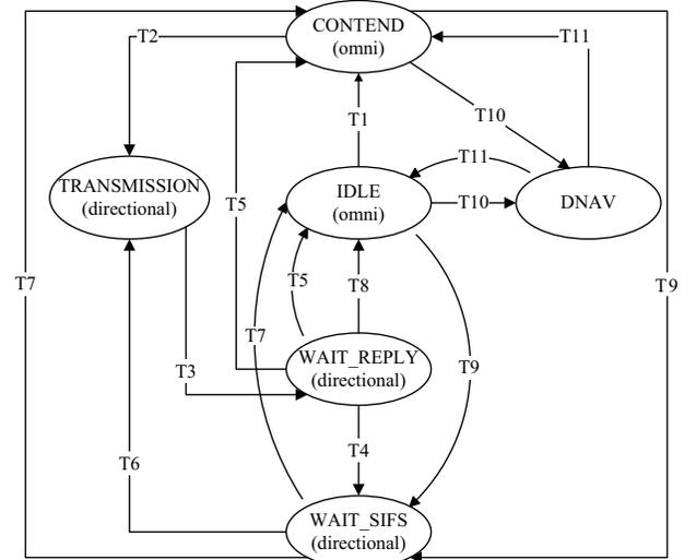
Fig. 4. State transition diagram of proposed MAC protocol.
