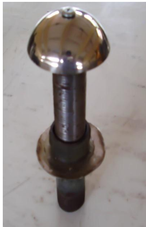
Fig. 6. Hyperperbolic mirror attached with a threaded pipe and socket.
