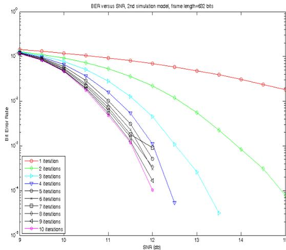
Fig. 12. BER vs SNR (dB) for the 2<sup>nd</sup> simulation model and a frame length of 632 bits
