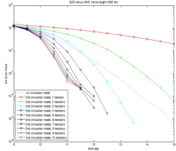
Fig. 13. BER vs SNR (dB) for the 1<sup>st</sup> simulation model (uses convolutional coding – dashed line) and the 2<sup>nd</sup> model (uses SCCC turbo coding) and a frame length of 1632 bits
