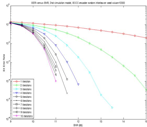
Fig. 17. BER vs SNR (dB) for the 2<sup>nd</sup> model and a SCCC encoder random interleaver seed value of 12000
