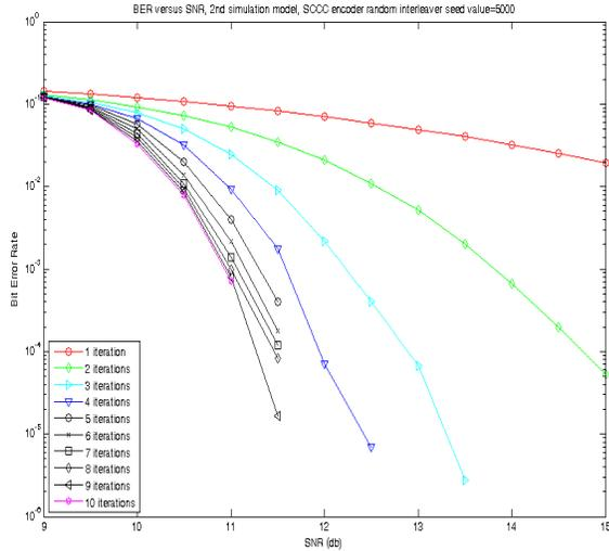
Fig. 16. BER vs SNR (dB) for the 2<sup>nd</sup> model and a SCCC encoder random interleaver seed value of 5000
