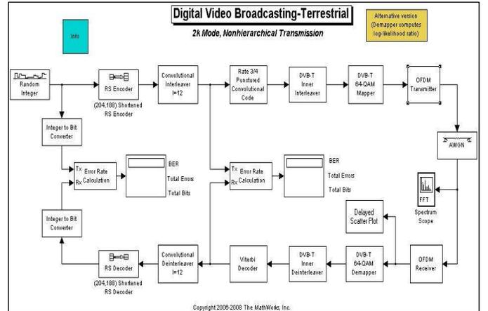
Fig. 6. Simulink 1<sup>st</sup> simulation model with convolutional and RS encoding-decoding
