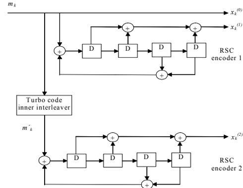
Fig. 2. UMTS PCCC turbo encoder
