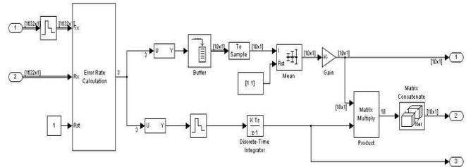
Fig. 9. Multiple iteration error rate calculation block
