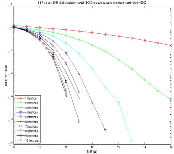
Fig. 18. BER vs SNR (dB) for the 2<sup>nd</sup> model and a SCCC encoder random interleaver seed value of 40000
