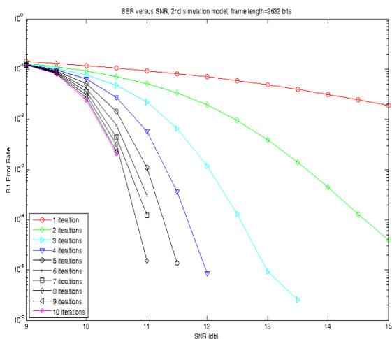
Fig. 14. BER vs SNR (dB) for the 2<sup>nd</sup> simulation model and a frame length of 2632 bits
