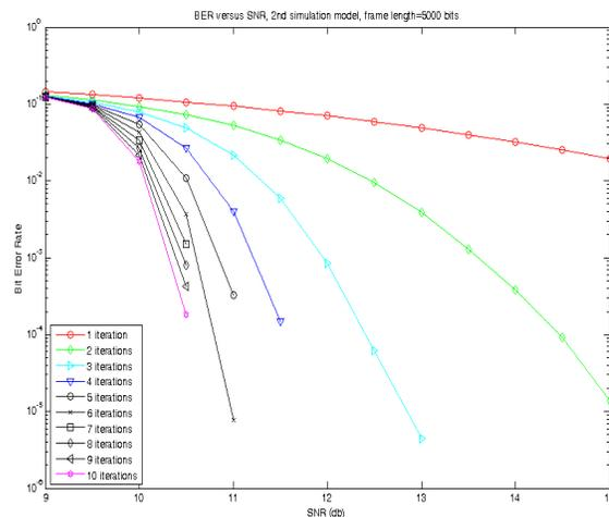
Fig. 15. BER vs SNR (dB) for the 2<sup>nd</sup> simulation model and a frame length of 5000 bits
