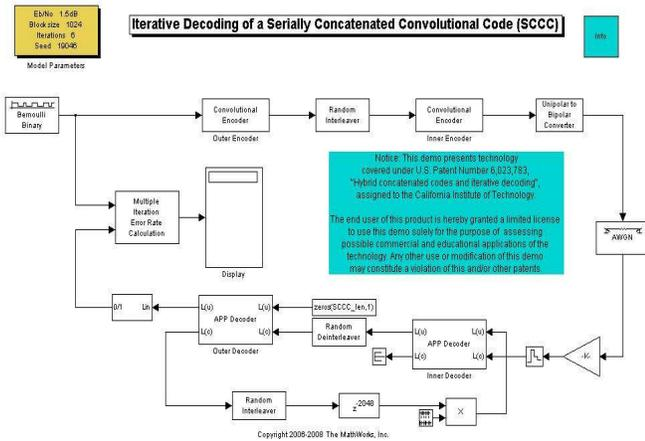
Fig. 7. Simulink SCCC encoding-decoding system
