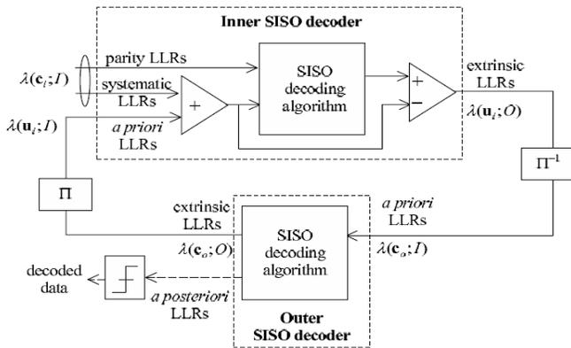
Fig. 5. SCCC turbo decoder [12]
