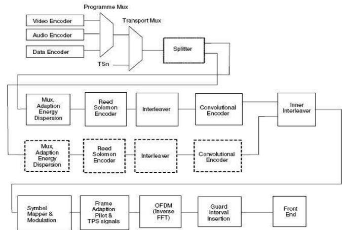
Fig. 1. DVB-T transmitter functional block diagram.
