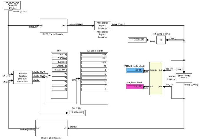
Fig. 8. Simulink 2<sup>nd</sup> simulation model with SCCC encoding-decoding
