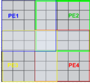
Fig. 8: 2D Illustration of pixel processing distribution amongst PEs
