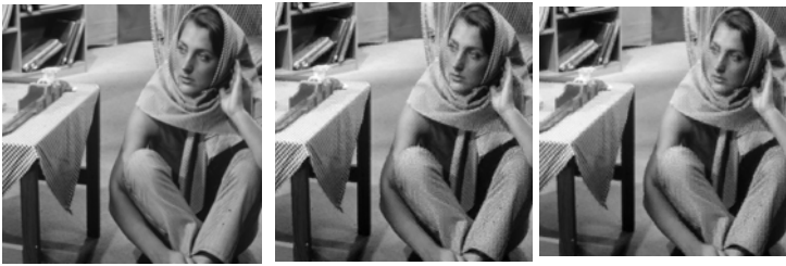
(a) (b) (c) Figure 6. (a)Original image, (b), (c) compressed images using BTC and AMBTC respectively
