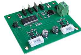
Fig. 6 Motor driver, 12v 2.8A Dual H-Bridge
