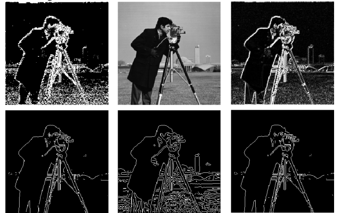
Figure 12 Edge detection comparison, Top, left to right: wavelet-based technique, original, MMW technique, Bottom, left to right: Sobel, Canny, Prewitt edge detectors.
