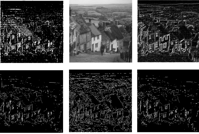
Figure 13 Edge detection comparison, Top, left to right: wavelet-based technique, original, MMW technique, Bottom, left to right: Sobel, Canny, Prewitt edge detectors.
