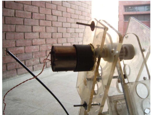
Fig.3 Third DC motor is used in the set up for moving the arm up and down.
