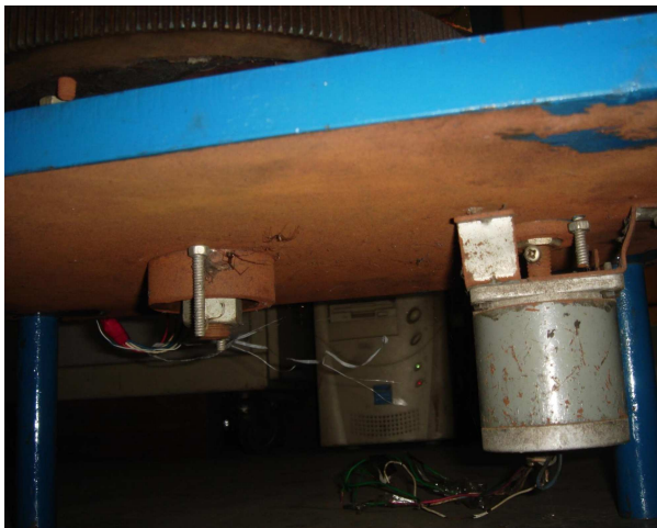
Fig.1 First DC motor is used in the set up to rotate the base.
