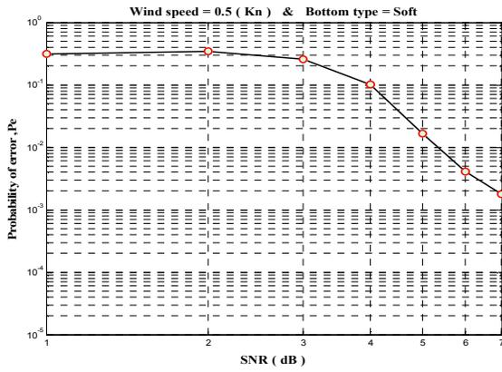
Fig. 10. Probability of error of detected symbols versus SNR under the condition of wind speed=0.5Kn, and soft bottom
