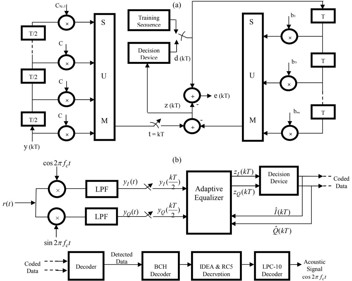
Fig. 5. (a): Decision Feedback Equalizer. (b): Block diagram and structure of the receiver
