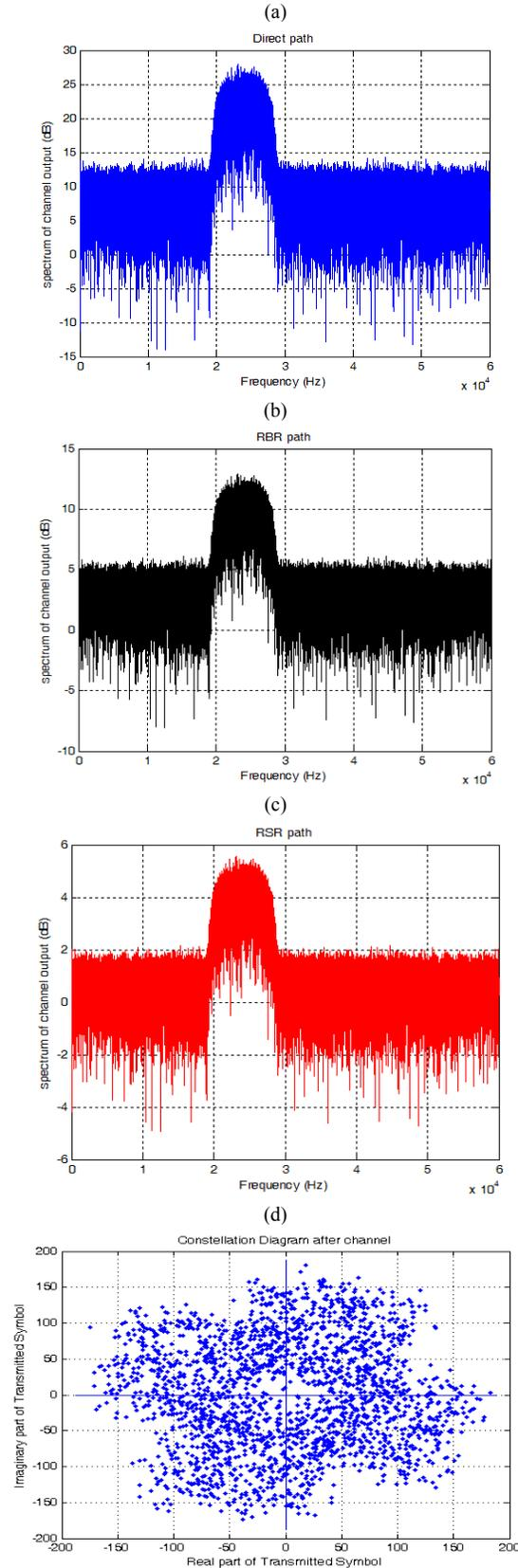
Fig. 9. Power spectrum density of the four special paths used in the simulation. (a): Direct Path (DP). (b): Refracted Bottom Reflected (RBR). (c): refracted Surface Reflected (RSR). (d): Refracted Surface Reflected Bottom Reflected (RSRBR).
