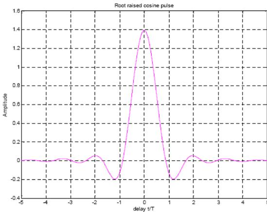
Fig. 2. Impulse response of the pulse shaping filter
