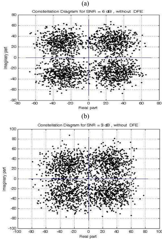
Fig. 11. The constellation diagram of symbols detected by the simple receiver that has no DFE in its structure
