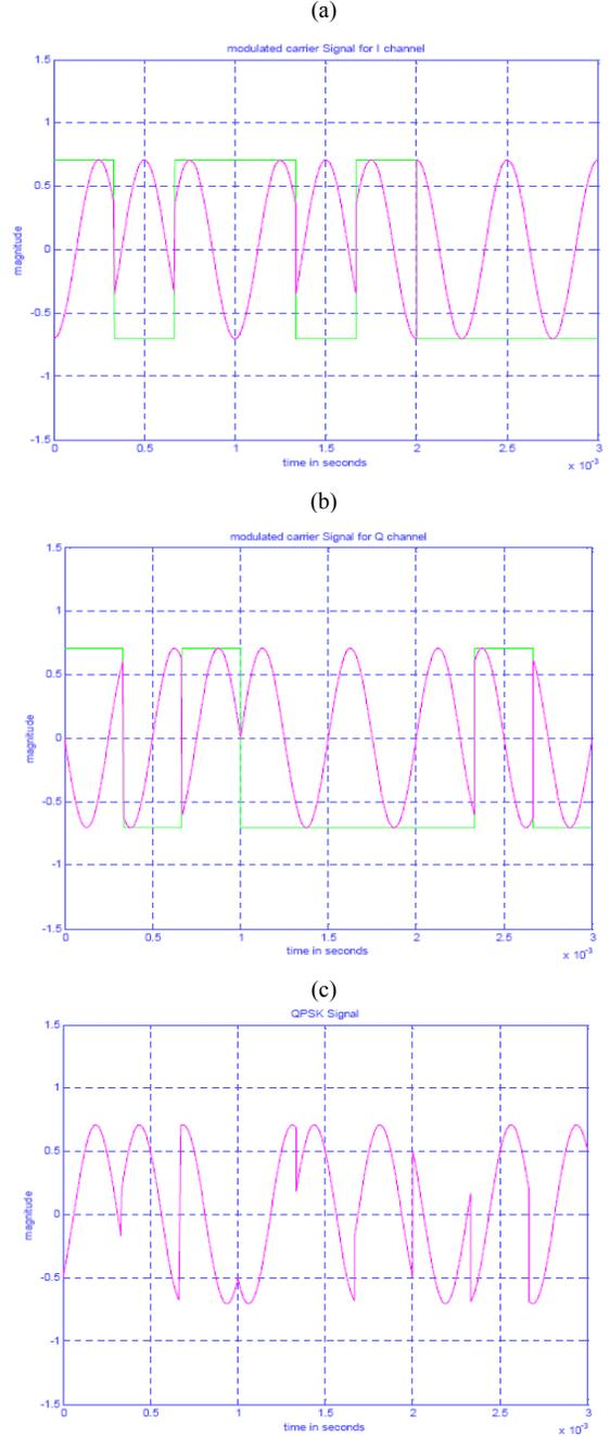
Fig. 3. (a). I channel - (b). Q channel (c). - QPSK signal
