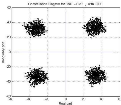
Fig. 12. The constellation diagram of symbols detected by the receiver that has a DFE in its structure for SNR=3 dB
