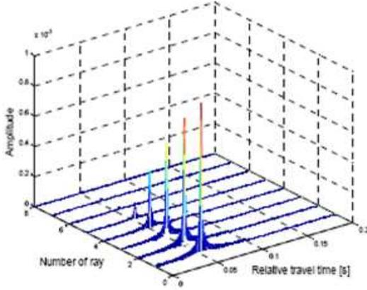
Fig. 4. Received signals from different paths of channel. In this model, channel has 8 paths. The first signal is for the direct path and the delays of other paths are calculated based on the travelling time of the first path.
