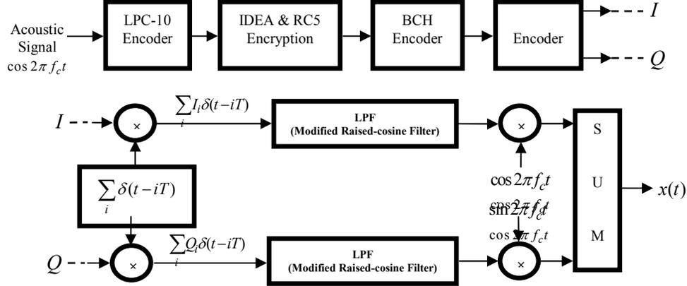
Fig. 1. Block diagram and structure of the transmitter.
