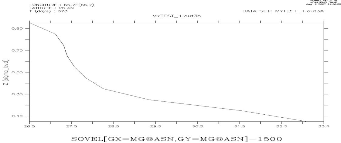
Fig. 6. a profile of sound speed variation with depth for the Strait of Hormuz, in  $56.7^\circ\text{E}$  (Lon) and  $25.4^\circ\text{N}$  (Lat). The water depth was 85m, and the ADCP measurement tool, belonging to the NOAA submarine, was placed at a depth of 10 m.
