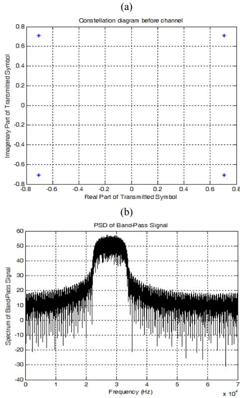
Fig. 7. (a): Constellation diagram of QPSK symbols. (b): power spectrum density of band pass signal before entering the channel
