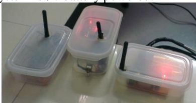
Fig. 15. The releasing Circuit is sending the parameters to the central circuit
